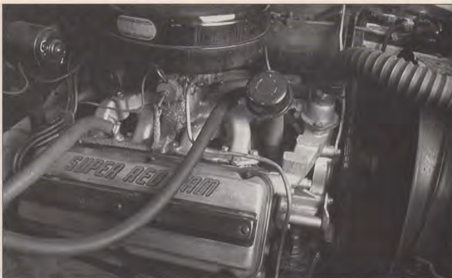
Fed by a two-barrel Stromberg, the Super Red Ram Hemi V-8 makes 183hp at 4,400 rpm.
